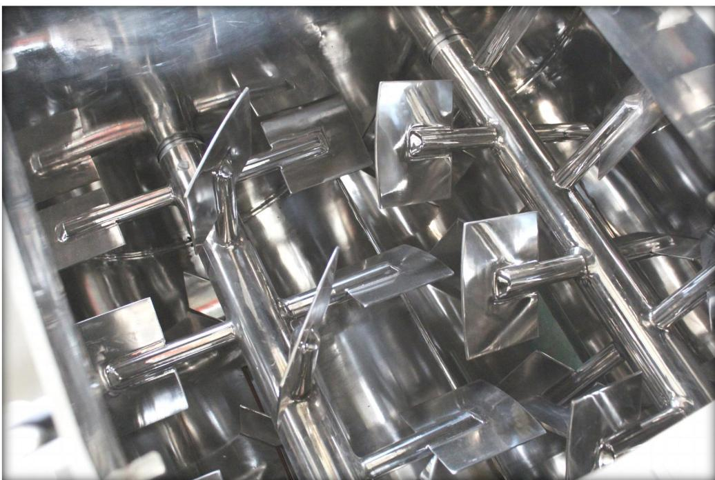
At this weightless zone, mixing of materials of different density is easy and fast because material particle can move freely and randomly, regardless of particle size and density. This brings a rapid and highly homogenous mixing.
