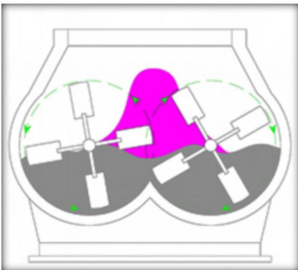
The PerMix PFB series Twin-shaft Paddle Mixer consists of paddles with special angles that are mounted on twin shafts in a "W" shaped trough. During operation, the two shafts are rotating in opposite direction.
