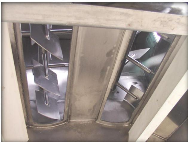
PerMix offers large Bomb Bay Door for fast and efficient discharge, also reducing the segregation as much as possible.
